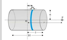
Magnetic field due to element dx at point P
